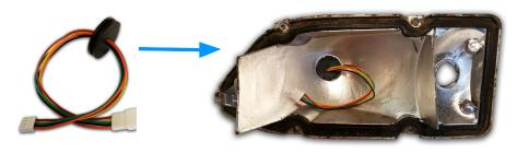
2. Wrap the rubber grommet around the wires and press it into the socket hole.
