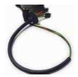
Be careful when handling the wires that are attached to the LED panel. The connection where the wires meet the LED panel are sensitive to prolonged bents.
