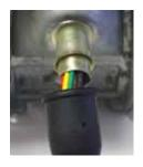
3. Slide the tube and body grommet over the wires. The tube ends should fit inside the ends of the boot and grommet for a sealed finish.
