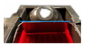
7. Cut away the remaining triangular plastic areas so that the light emitted from the LED panel will not be blocked. Also make sure that the cut away area does not stick up over the housing ledge.
