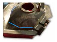
**4.** Mark the lower bucket, next to the reverse light socket, level with the housing ledges.
