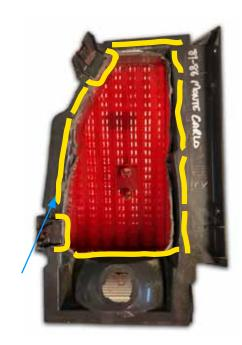
3. Lay the LED panel in place and firmly press it down. hold down the LED panel and tape it in place. It will need 24 hours to dry. Run a final bead of silicone across the bottom of the LED panel to close off the remaining gap.
