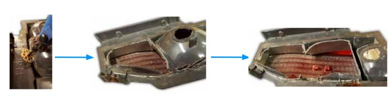
6. Be sure that the cut at the bottom of the bucket is even with the housing ledge.
