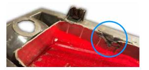
**8.** There are 2 housing mounts molding into the housing. In order for the LED panel to sit proper and flush you will need to trim back some of the raised plastic like shown below.
