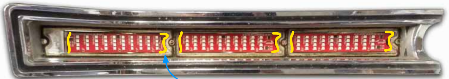
Carefully apply the silicone so you do not cover up any of the LEDs.
