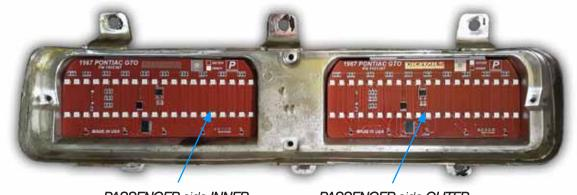
PASSENGER side INNER PASSENGER side OUTER PASSENGER side tail light housing.
