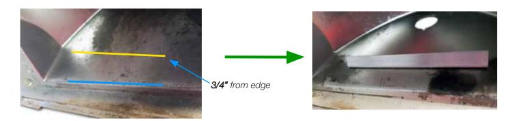
2. Looking at the **UPPER** portion of the housing light pocket. Measure back 5/8" from the edge and mark. Then mount the single bracket right behind the mark.
