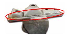
**3.** Cut into the remaining sides of the housing buckets. This will loosen them to the point where they will easily separate from the lens.
