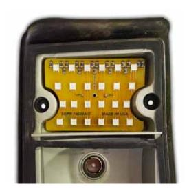
Take the brake light(red) LED panel and twist in the light plug into the bottom light socket. Test fit the LED panel. Once you are satisfied with the fit peal off the remaining protective strips and attach the LED panel.
