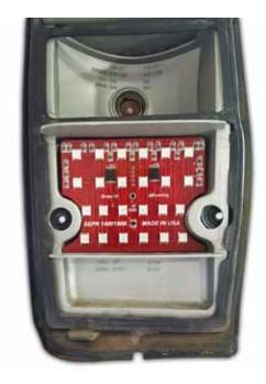
Screw the lens back onto the light housing and reinstall the light housing assembly.
