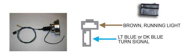
Male blade terminals and connectors are included in case your factory front light harness connector is missing or damaged.
